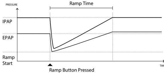
If ramp is activated with AVAPS enabled, it will reduce the maximum pressure support capability to IPAP Min or PS Min and ramp to the IPAP Max or PS Max over the ramp time period. During the ramp period, the prescribed tidal volume may not be achieved.
