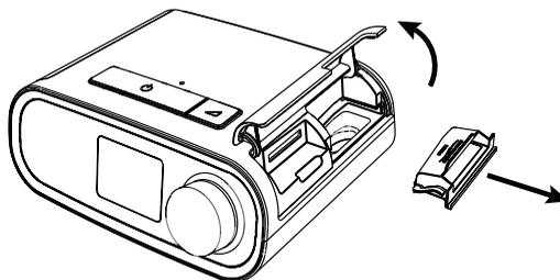
2. If applicable, place a clean, reusable blue pollen filter (1) on top of a new, optional disposable light-blue ultra-fine filter (2) and firmly snap them together.
